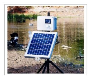
Eureka TS2 telemetry systems – the TS2 telemetry system installs in the field in minutes with no user programming; you can view data at any Internet connection. The TS2 uses your choice of cellular or satellite communications for high reliability at lowest cost.
